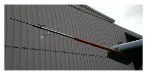
Figure 1: NACA Air Data Boom Design with Flow Angle Vanes on the UTSI Cessna 210 right wingtip.
