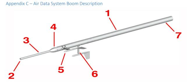
Figure 25: SpaceAge Control 100400 Mini Air Data Boom 3D model
