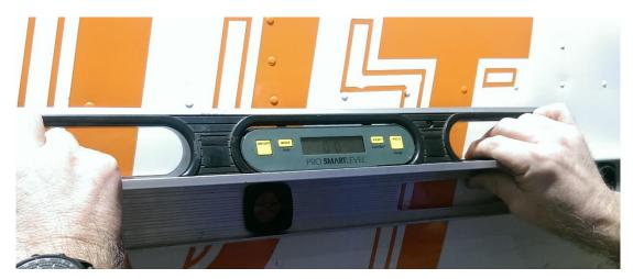
Figure 13: Aircraft water level reference line. The ADS Boom aligned with this reference line; the INS unit has a 0.1° offset from this reference line.
