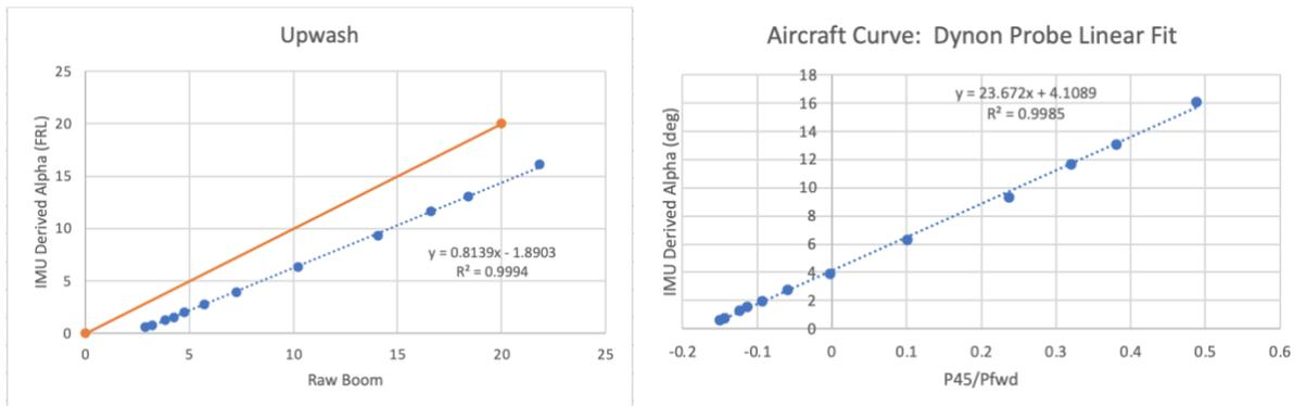
**Figure 16. Representative IMU Derived Upwash and AOA Calibration Curves**
