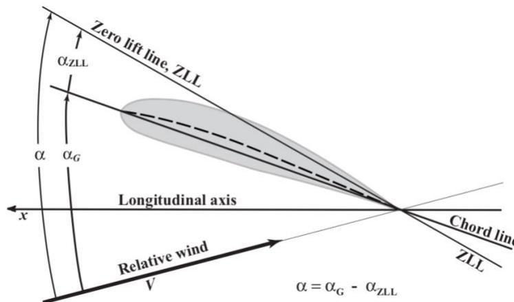
Figure 7. Angle of Attack.<sup>4</sup>
