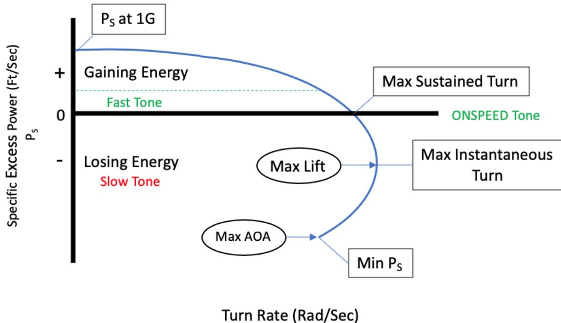
**Figure 6. Specific Excess Power vs Turn Rate**
