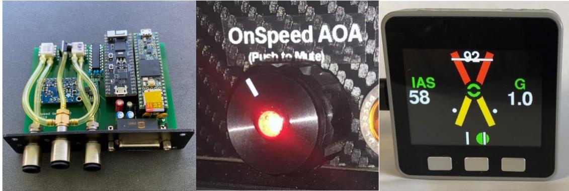
**Figure 1: Gen 2 Hardware: Box, Control Switch and Optional Energy Display**
