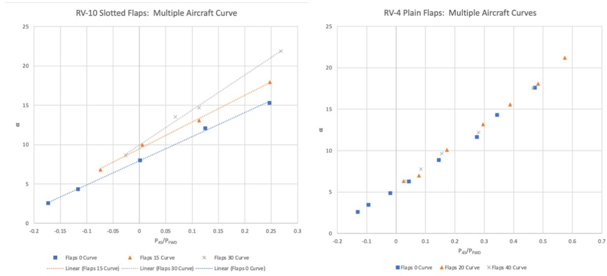
**Figure 13. Type of Flap, Effect on Aircraft Curves**
