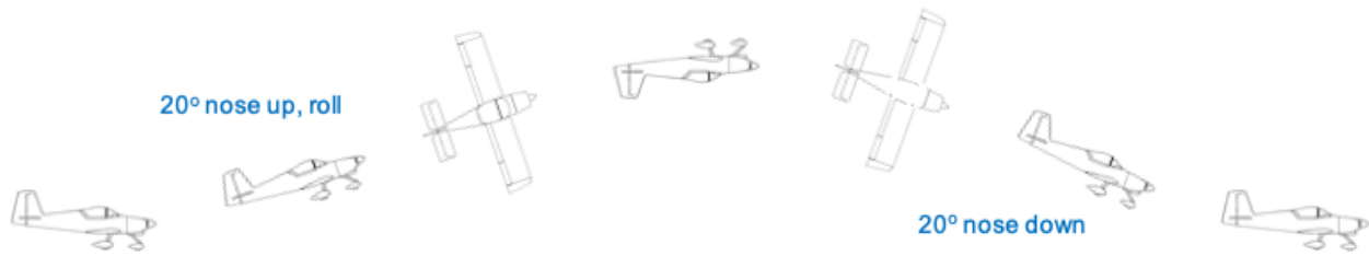
Figure 5. “Angles = angles” Rule Applied to a Simple Aileron Roll
